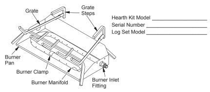
Figure 1 - Product Identification (Dual Burner Shown)
